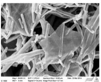
Figure 1 – FESEM image of 3D composite carbon felt with free-standing RGO basal planes(left) and Ppy-HS/GO (right).
